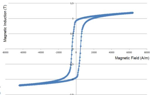
Fig. 8 – Hysteresis loop of sintered pure iron.
