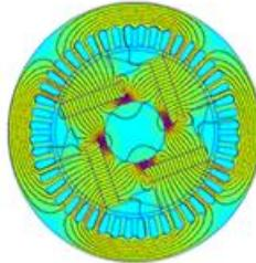
Fig. 18 - Machine simulation with rotor of embedded magnets from M15 steel sheet - Flux lines in the longitudinal plane of the machine.
