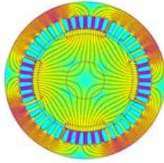
Fig.16 – Machine simulation with rotor of straight poles from Fe-2%P sintered - Flux lines in the longitudinal plane of the machine.
