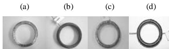
Fig. 3 Sample preparation steps: (a) isolating (b) secondary winding, (c) isolating and (d) the primary winding
