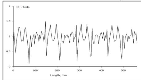
Fig. 9 - Machine simulation with rotor of salient poles from M15 steel sheet - Air-gap flux density.
