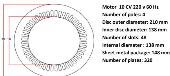
Fig. 5 – Schematic of machine stator sheets.
