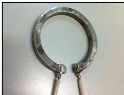
Fig.4 – Segmented ring for measuring electrical resistivity.
