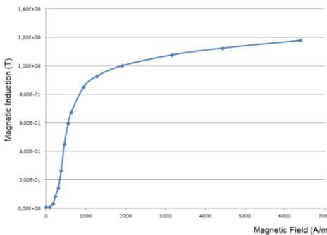
Fig. 7 – Magnetization Curve sintered pure iron.
