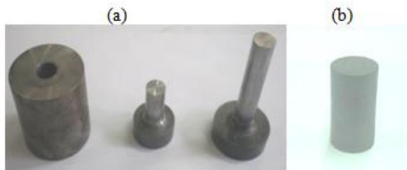
Fig. 2 - Samples in the form of cylinder - (a) Die - (b) Specimen.
