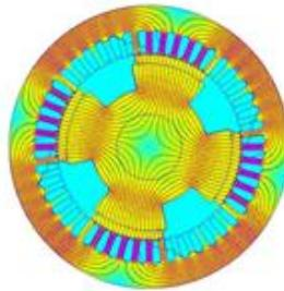
Fig. 10 - Machine simulation with rotor of salient poles from M15 steel sheet - Flux lines in the longitudinal plane of the machine.
