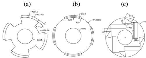
Fig. 6 – Topology of rotors studied - (a) salient poles with magnets on the surface of the saliences - (b) straight poles with magnets on the rotor surface - (c) embedded magnets within the rotor.
